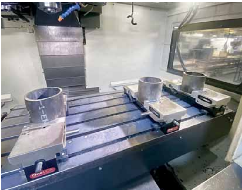
Circular and other non-prismatic parts are clamped in the OneLOKs in soft aluminium jaws machined to match their shape. The jaw sets can be exchanged in seconds.
