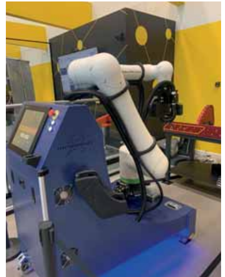
An aerospace drilling cell developed by Electroimpact and featuring a FANUC CRX-25iA cobot, will demonstrate accessible and cost-effective pre-validated drilling functionality for the aerospace sector.
