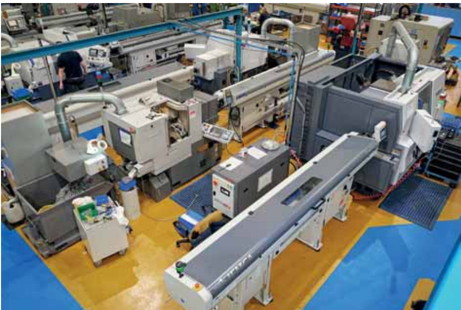
A view of Apel's shop floor, showing the Citizen Cincom lathes and the Miyano in the foreground.
