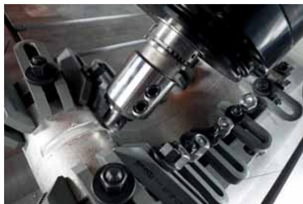
Robot-based FSW technology is particularly suitable for 3D welding, a challenge in production.
