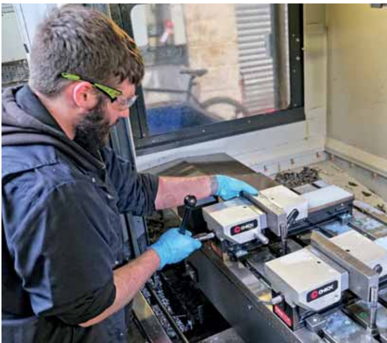
Archway Engineering programmer-operator Ben Jaine setting up a new batch of components in the three Chick OneLOKs on the table of the Leadwell VMC, ready for machining in one continuous CNC cycle.
