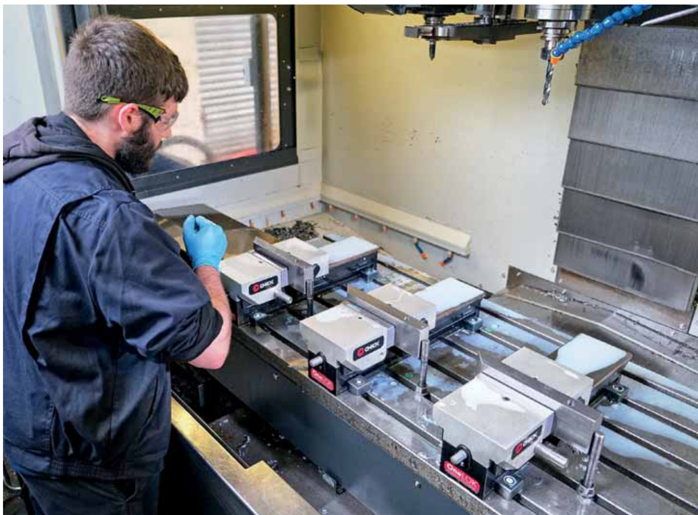
Archway Engineering programmer-operator Ben Jaine setting up a new batch of components in the three Chick OneLOKs on the table of the Leadwell VMC, ready for machining in one continuous CNC cycle.
