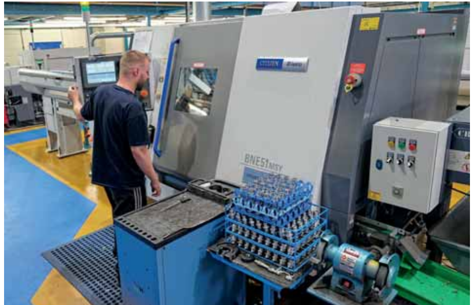
The Miyano BNE-51MSY fixed-head lathe is seen here producing stainless steel aerospace components.
